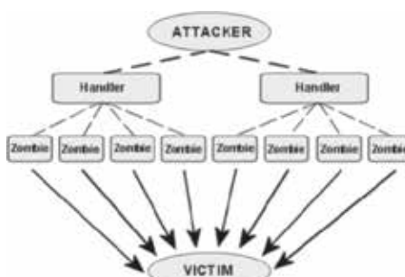
Figure 1: Architecture of DDoS attack.
